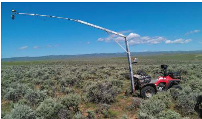
An ATV is mounted with a DSLR camera on an extended boom to shoot high-resolution images of ground cover. Photo courtesy of Open Range Consulting, Inc.
