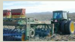
A Lawson aerator is a large, weighted drum pulled behind a tractor that crushes sagebrush and impacts the soil surface.
