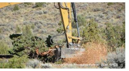
Mastication is one method of removing encroaching trees. Heavy machinery, equipped with special masticators, grinds up encroaching trees where they grow.
